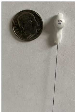
Nanotag next to a dime for size reference. Photo by Stephen Brenner
